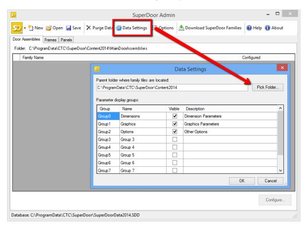
The content folder can be placed in any location accessible to all users; however the subfolder structure must remain unmodified.
